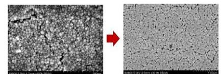
Calendering, where the print is squeezed between rollers, is also used in post processing to compact the ink and further improve performance.
