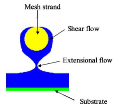
An example of the relationship between rheology and printability is given from the ARPLAE case study of a model screen printing ink (an exemplar project of the EPSRC Centre for Innovative Manufacture of Large Area Electronics)
